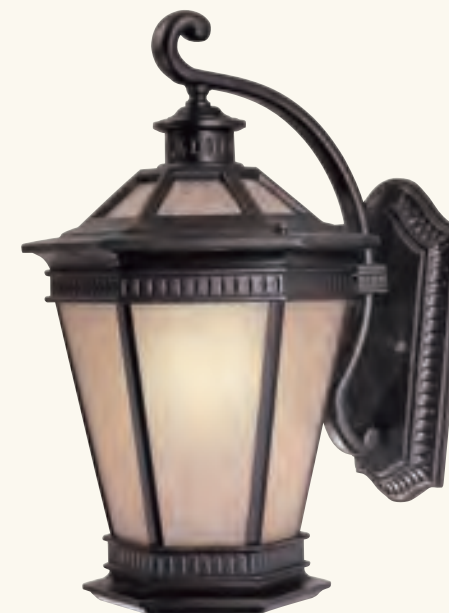
9790-68 1–13W self ballasted compact fluorescent lamp with GU24 base included. ENERGY STAR® qualified. 8" W x 13 1/4" H x 9 1/4" Ext. Backplate: 5 1/2" W x 8 1/4" H
